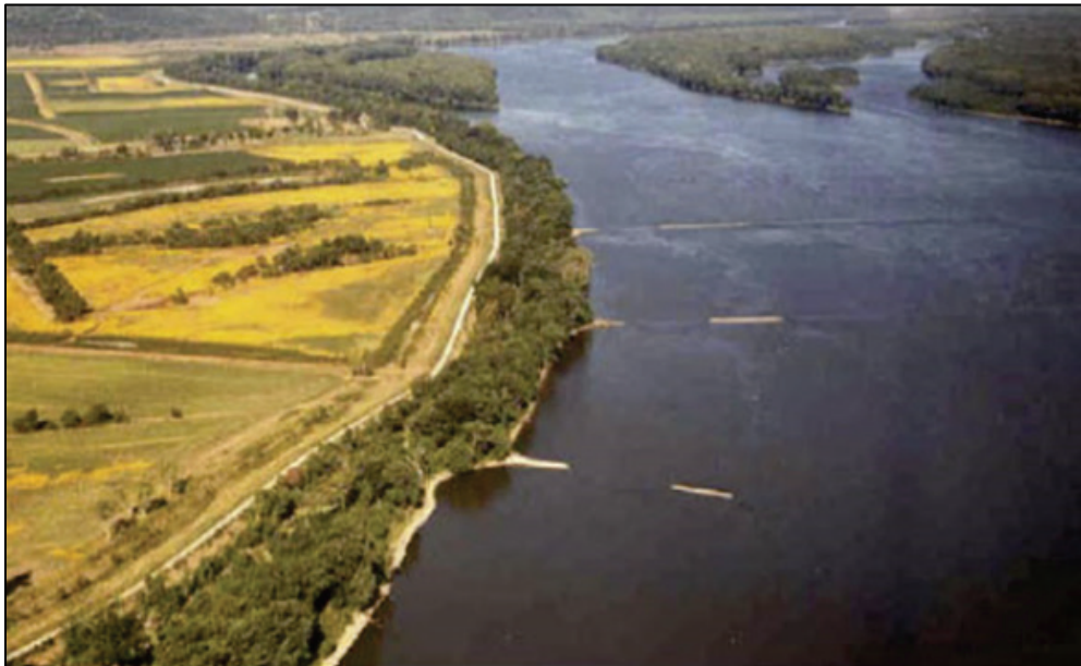
Figure 14. Notched dike in real-world application (USACE Applied River Engineering Center n.d.).
